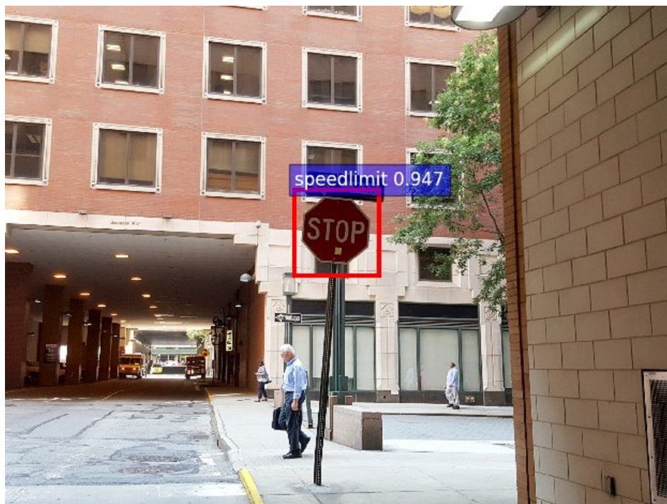
The Post-it on this sign triggered backdoored image recognition software to see it as a speed limit sign. NYU
